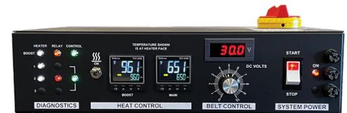
Lo-E series dryers have a dual zone heat control, with a boost zone to quickly reach cure temperature. This makes it GREAT for inkjet curing!
