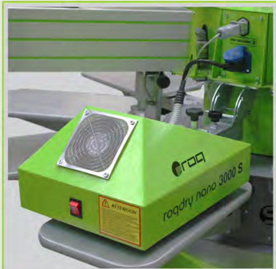
:: NANO FLASH CURE UNIT EMBEDDED IN THE STRUCTURE
