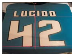
Lines used to position name and numbers on a heat transfer press
