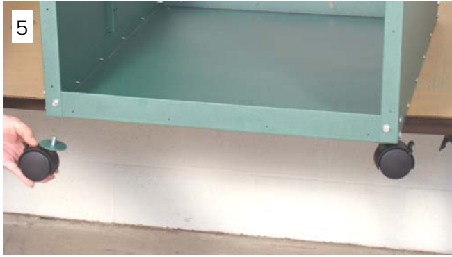
5) Install all (4) casters using a green washer under the Bottom Panel, and a 3/8" washer, lockwasher, and nut on top. Tighten with a 9/16" wrench.
