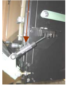
GAS SPRING. Shown inserted.
